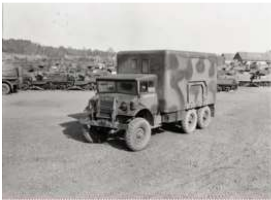
Canadian Military Pattern truck in version used for mechanical repairs. Chevrolet Model C60X, 3-ton, 6 wheel lorry. Canadian designed and built in Oshawa, Ontario. England, 19 March 1944.
